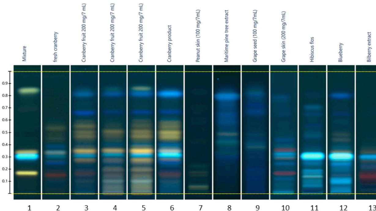
**Figure 4: HPTLC analysis of cranberry, related and adulterating species.** Lane 1: rutin, chlorogenic acid, hyperoside, and quercetin, with increasing Rf value; Other lanes as indicated above. Stationary phase: silica gel 60 F254; Mobile phase: toluene-water-formic acid-ethyl formate (3:6:8:60); Detection: Natural product reagent, viewed using UV light at 366 nm. Image provided by Camag AG; Switzerland.
