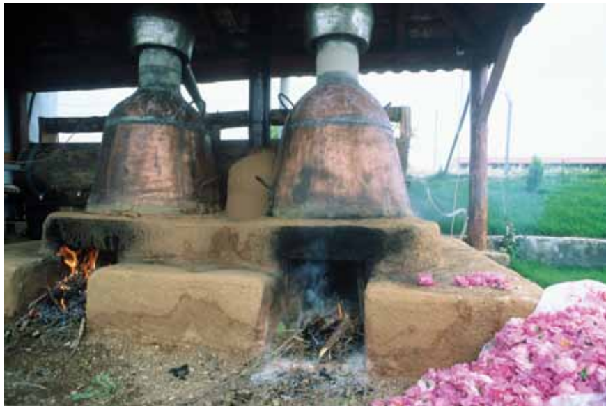
Village-type rose oil distillation facility in Turkey.
